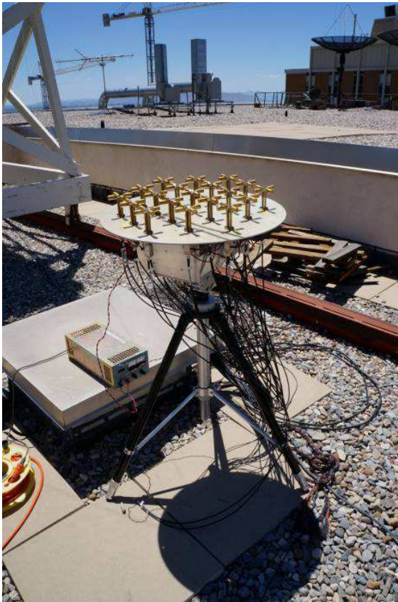
(a) The 19 element PAF used to test the xRTB.
